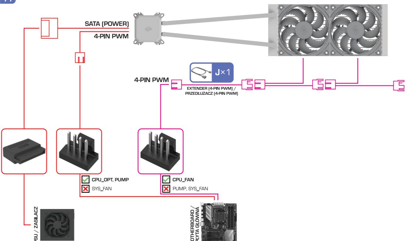
**!** EN: The red line shows how to correctly connect the pump. Connect the power to a SATA plug and control signal to a 4-pin fan connector. Configure your motherboard for speed control in PWM mode (consult the motherboard manual for details).
