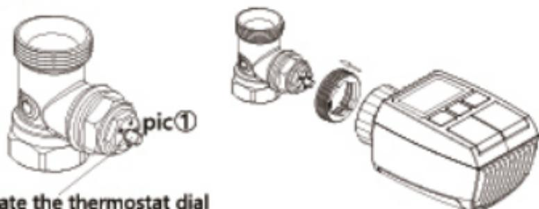
**Rotate the thermostat dial to the maximum value**
